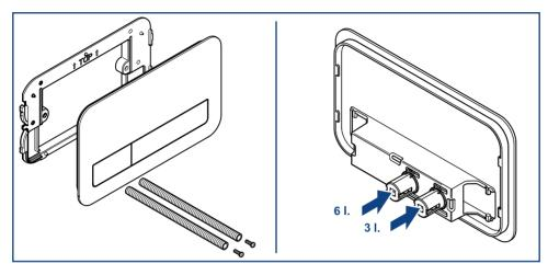
1. Screw the carrier plate in place.
