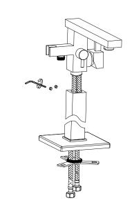
3. Create a chamber in the floor following the above measure with G1/2 male connectors for water net.
