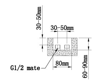
**4.**Insert the sliding cover on square pole, insert the flexible hose's nuts throw the fixing base and connect the G1/2 nuts with the water net connectors fixing tight by key.
