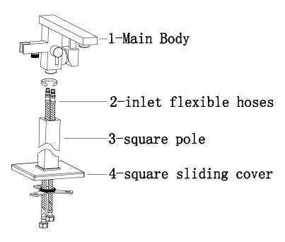
2. Match the square pole with the main body, fix together turning the 2 screws on rear with the key.
