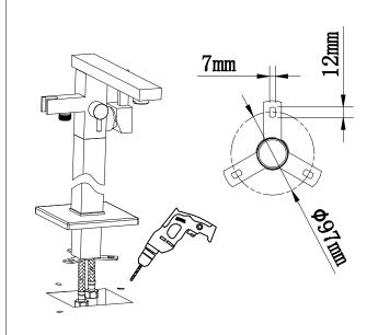
6. Insert the fixing bolts and fix tight in the floor.
