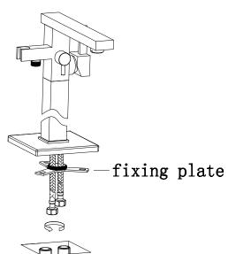
**5.** Adjust the complete to get correct position ,then drill to fix the base plate.
